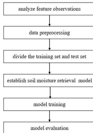
Fig. 3: Flowchart of the soil moisture retrieval algorithm.
