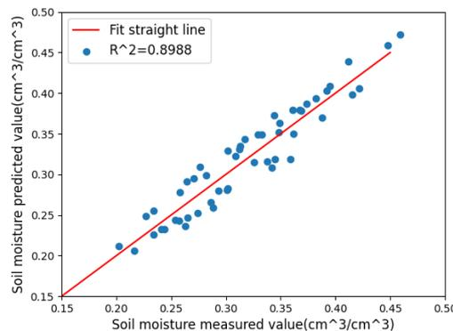
Fig. 6: Correlation between the predicted value of the Elman model and the measured soil moisture value.
