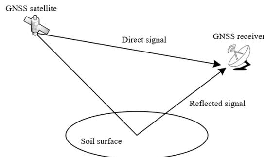
Fig. 1: GNSS signal superposition phenomenon.
