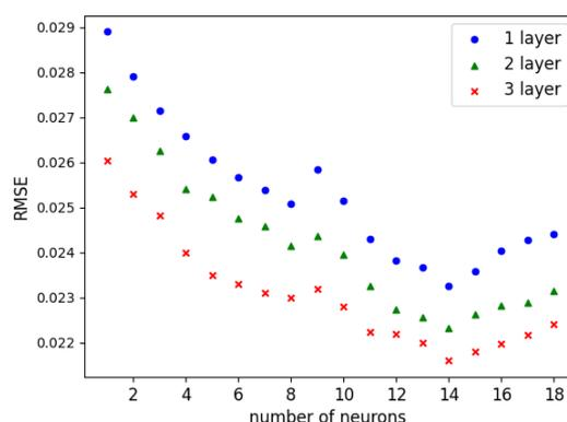
Fig. 4: RMSE of the predicted soil moisture with different number of hidden layers and neurons.
